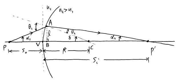
Point-like object (light source) P and the center of curreture of the spherical surface define the axis of such a simple optical system, namely, PC. When the light come emitted from P forwards the surface is restricted to be small so that 2 << R, So, Si in magnihile, all angles such as d., d. S, O., O. are small. This is the condition of paraxial approximation
