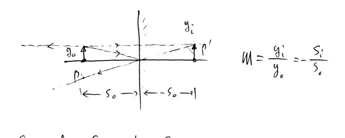
Focal points of a spherical minor:
