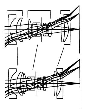
Figure 1. 21.4--29.5 mm f/3.6--f/4.6 zoom lens for a compact 35-mm camera.
