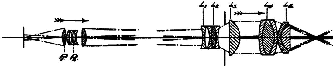
**Figure 1.** Microscope system discussed by H.D. Taylor, which includes a five element flat field anastigmatic objective and an inside focus wide-angle eyepiece. The eyepiece consists of five groups of lenses, L1 through L5.<sup>11</sup>
