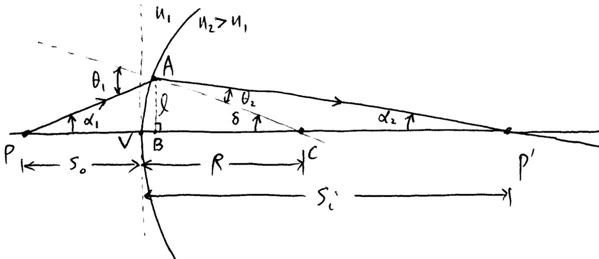
Point-like object (light source) P and the center of curvature of the spherical surface define the axis of such a simple optical system, namely, PC.
