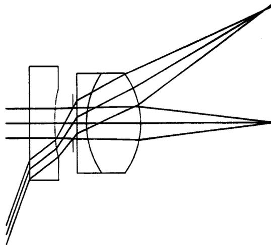
**Figure 1.** 1.0 mm EFL. 140° full field-of-view, f/4.025, endoscope objective.
