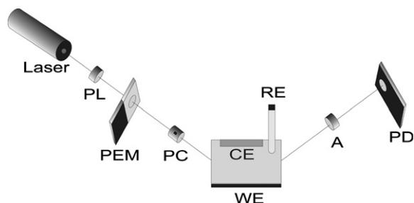
Fig. 1. Sketch of the electrochemical cell and optical set up for the oblique incidence reflectivity difference experiment. Laser: 15 mW He–Ne laser; PL: Glan-Thompson polarizers; PEM: photoelastic modulator (Hinds Instruments); PC: Pockels cell; CE: counter electrode; RE: reference electrode; WE: working electrode (Cu/Au/glass); A: analyzer; PD: biased silicon photodiode.
