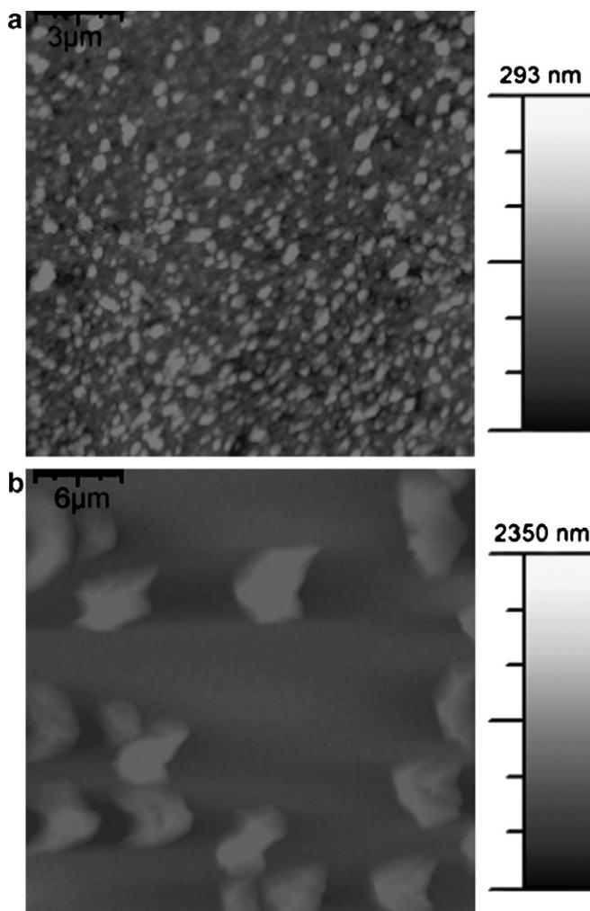
Fig. 8. (a)  $15 \times 15 \mu\text{m}$  in situ AFM image of islands formed by Pb deposition at  $E = -0.62$  V in 100 mM  $\text{HClO}_4 + 1$  mM  $\text{Pb}^{2+}$  electrolyte; (b)  $30 \times 30 \mu\text{m}$  in situ AFM image of islands formed by Pb deposition at  $E = -0.62$  V in the same electrolyte + 20 mM  $\text{KCl}$ .
