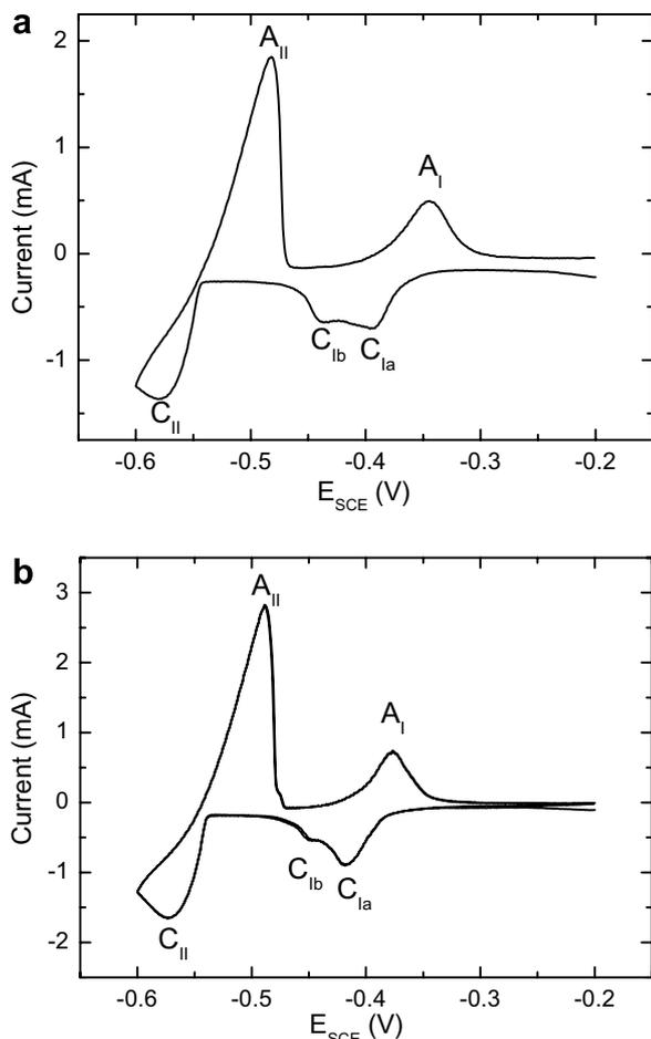
Fig. 2. Cyclic voltammograms for a (111)-textured polycrystalline Cu substrate measured in: (a) 100 mM  $\text{HClO}_4$  + 1 mM  $\text{Pb}(\text{ClO}_4)_2$ ; (b) 100 mM  $\text{HClO}_4$  + 1 mM  $\text{Pb}(\text{ClO}_4)_2$  + 20 mM  $\text{KCl}$ . The scan rate was  $10 \text{ mV s}^{-1}$  and all potentials are quoted with respect to SCE.
