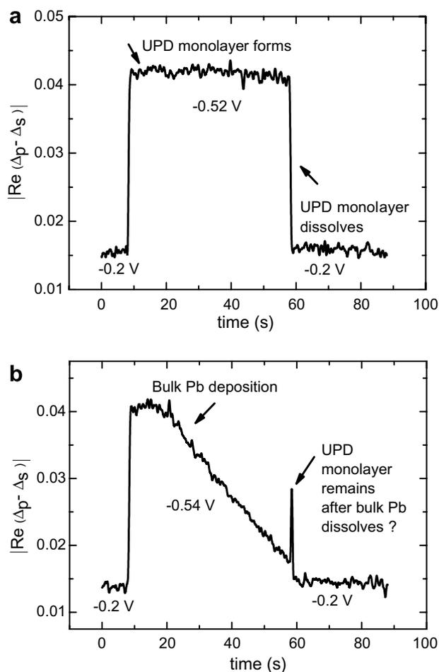
Fig. 5. OI-RD signal  $|\text{Re}\{\Delta_p - \Delta_s\}|$  (not normalized) recorded when stepping the Cu substrate potential (a) from  $E = -0.2 \text{ V}$  to  $E = -0.52 \text{ V}$  for  $t = 50 \text{ s}$  (UPD) and (b) from  $E = -0.2 \text{ V}$  to  $E = -0.54 \text{ V}$  for  $t = 50 \text{ s}$  (OPD). The electrolyte was  $100 \text{ mM HClO}_4 + 1 \text{ mM Pb}(\text{ClO}_4)_2 + 20 \text{ mM KCl}$ .
