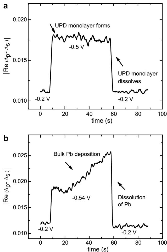
Fig. 3. OI-RD signal  $|\text{Re}\{\Delta_p - \Delta_s\}|$  (not normalized) recorded when stepping the Cu substrate potential (a) from  $E = -0.2 \text{ V}$  to  $E = -0.5 \text{ V}$  for  $t = 50 \text{ s}$  (underpotential deposition – UPD) and (b) from  $E = -0.2 \text{ V}$  to  $E = -0.54 \text{ V}$  for  $t = 50 \text{ s}$  (overpotential deposition – OPD). The electrolyte was 100 mM  $\text{HClO}_4$  + 1 mM  $\text{Pb}(\text{ClO}_4)_2$ .
