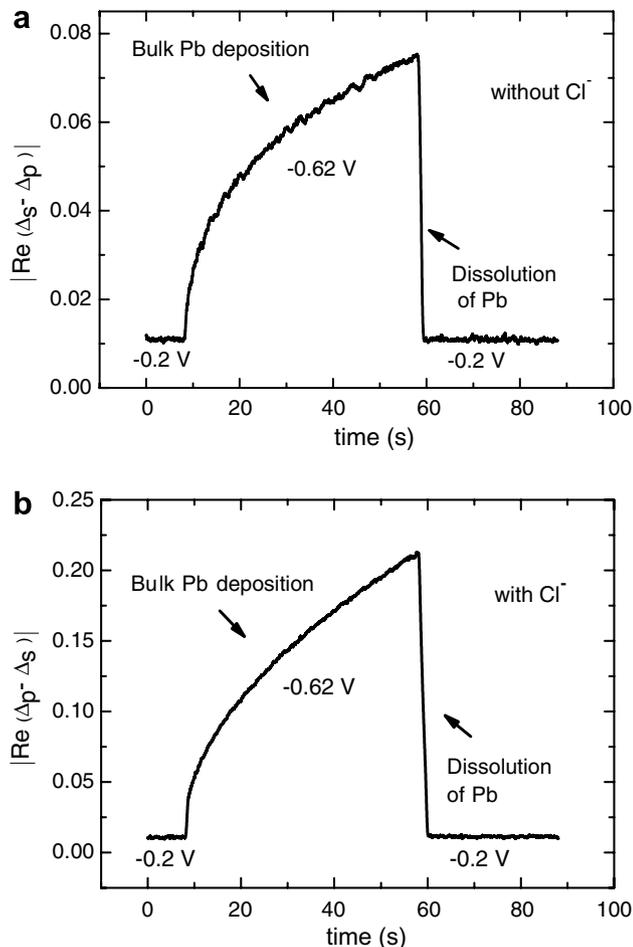
Fig. 7. OI-RD signal  $|\text{Re}\{\Delta_p - \Delta_s\}|$  (not normalized) recorded when stepping the Cu substrate potential from  $E = -0.2$  V to  $E = -0.62$  V for  $t = 50$  s (a) in 100 mM  $\text{HClO}_4 + 1$  mM  $\text{Pb}(\text{ClO}_4)_2$  and (b) in 100 mM  $\text{HClO}_4 + 1$  mM  $\text{Pb}(\text{ClO}_4)_2 + 20$  mM  $\text{KCl}$ .
