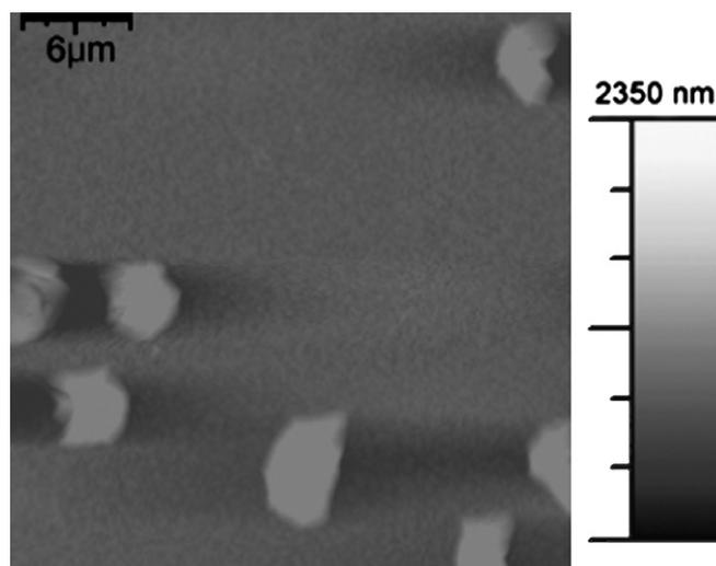
Fig. 6.  $30 \times 30 \mu\text{m}$  in situ AFM image obtained in  $100 \text{ mM HClO}_4 + 1 \text{ mM Pb}^{2+} + 20 \text{ mM KCl}$  electrolyte during growth at  $-0.54 \text{ V}$ .
