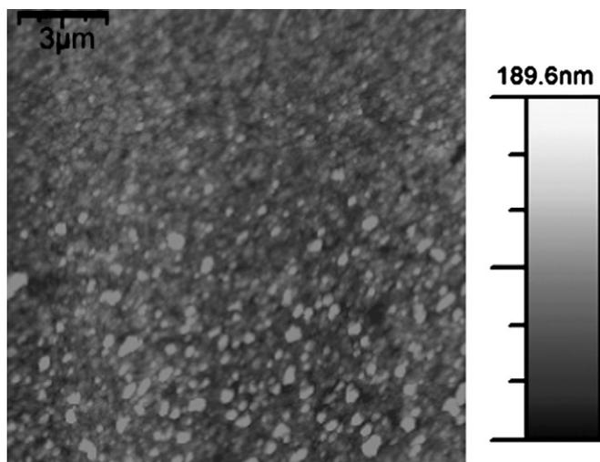
Fig. 4.  $15 \times 15 \mu\text{m}$  in situ AFM image obtained in  $100 \text{ mM HClO}_4 + 1 \text{ mM Pb}^{2+}$  electrolyte during growth at  $-0.54 \text{ V}$ . The island size increases from the top of the figure (start of scan) to the bottom (end of scan) as growth proceeds.
