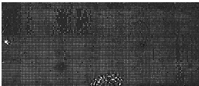
Figure 3. Surface coverage of 9,216 printed OBOC compounds on an epoxy-coated glass slide, deduced from the change in OI-RD image of microarray D after BSA blocking treatment and Eq. (2) in the main text. The average coverage in each spot is close to 50% of the printed area.
